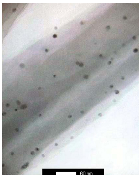
Fig. 9. TEM image of electrospun cellulose acetate nanofibers containing silver nitrate after irradiation with UV light at 365 nm for 240 min (scale bar, 60 nm) (from ref. [50] with permission).
